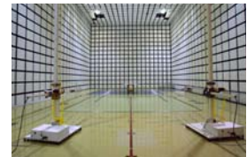
EMC testing in a 10 m wave anechoic chamber
