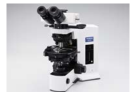
Phase-contrast polarization microscope for asbestos detection
