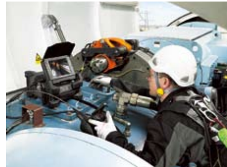
An IPLEX-FX industrial videoscope in use at a wind power generation facility in New Zealand
