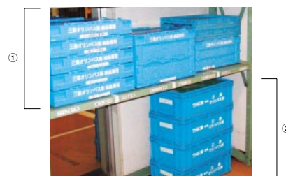
Special Returnable Box Used for Packaging ① Folding plastic box. The shock absorbent-material inside is returnable. ② Plastic cardboard. The shock-absorbent material is for exclusive use.
