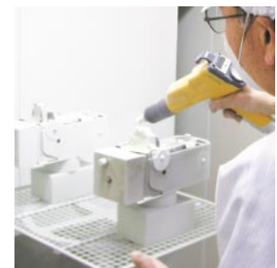
Powder Painting of Components for Microscopes
